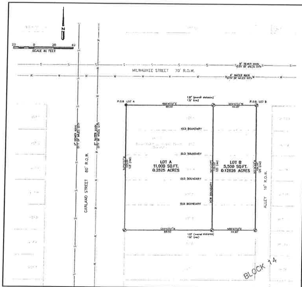
Figure 1: Excerpt of proposed Lot A and Lot B per the draft amended plat
