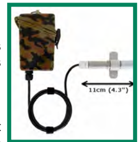
This infrared trail counter by TRAFx is an example of a permanent device with a web-based software solutions to view and manage the data.
